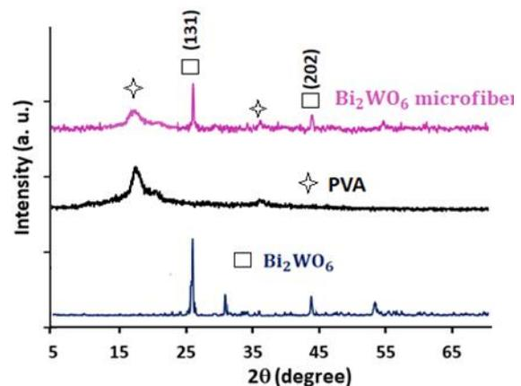
Fig.2. XRD patterns of the prepared samples
