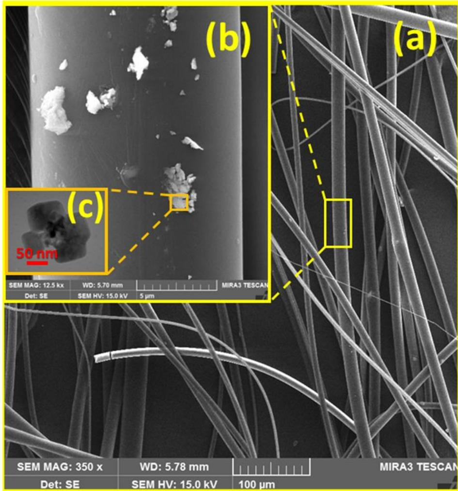
**Fig.3.** (a)FESEM image of the prepared  $\text{Bi}_2\text{WO}_6$  microfiber with (b)inset FESEM image in different scale, and (c)TEM image of the pure  $\text{Bi}_2\text{WO}_6$  nanopowders.
