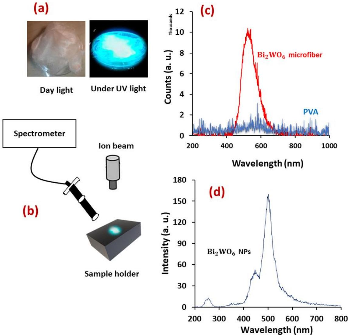
**Fig.4.**(a) Photos of luminescence properties of the prepared sample under UV light, (b)IBIL measurement setup, (c)IBIL spectrum of the neat PVA as background and prepared Bi<sub>2</sub>WO<sub>6</sub> microfiber, and (d)PL spectrum of the pure Bi<sub>2</sub>WO<sub>6</sub> NPs under 270 nm excitation wavelength at room temperature.
