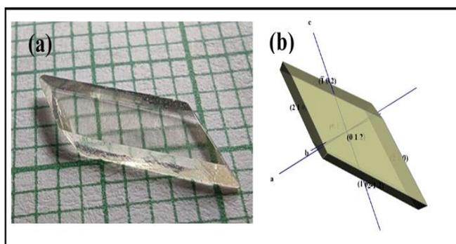
Fig. 2. (a) As grown BCNB single crystal and (b) its Morphology.
