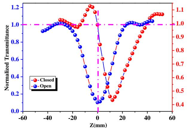
Fig. 6. Open and Closed aperture spectrum of BCNB.
