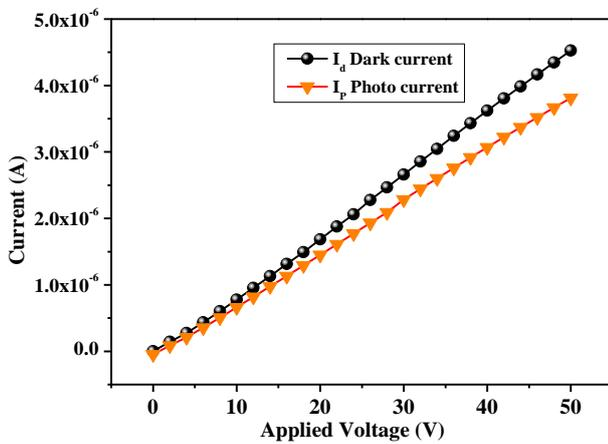
Fig. 5. Photoconductivity of BCNB crystal.
