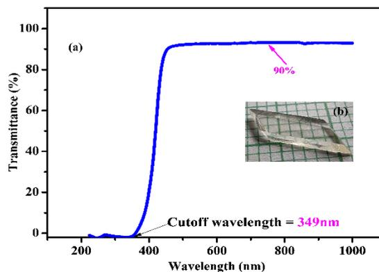
Fig. 4. (a) UV-Visible-NIR transmission spectrum of BCNB and (b) the photograph of BCNB sample (inset).
