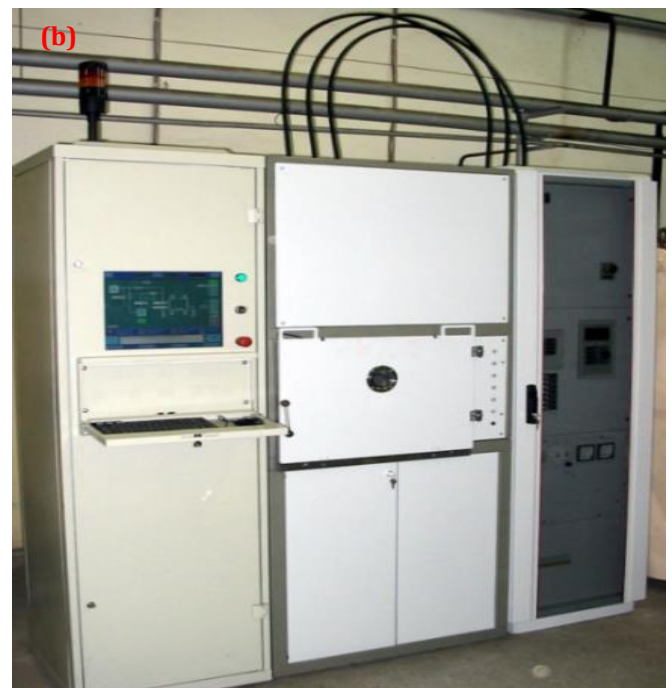
Fig. 1. The installation for the PEBI including (a) the RITM-13 for with short pulse duration and (b) the SOLO with a long pulse duration
