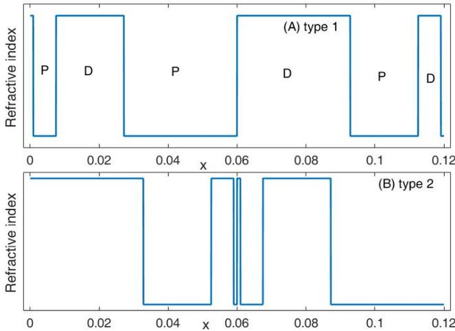
Fig. 1. Variation of the refractive index n as a function of the position x. each layer is devoted to a material kind. Layers alternatively composed from plasma with electron density  $n_e$  and dielectric material with refractive index  $n_1$ . P and D indicate the plasma and dielectric layers, respectively. Two configurations of the Pascal plasma photonic crystals are presented in panels (A) and (B)
