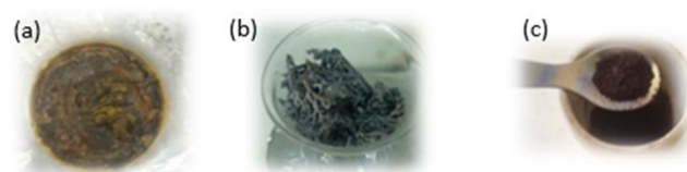
Fig. 1. Schematic representation of the sol-gel synthesis of \text{BaFe}_{12}\text{O}_{19} via the self-combustion reaction: (a) solution-to-gel transition, (b) auto-combustion at 300 °C, and (c) final powder obtained after annealing.
